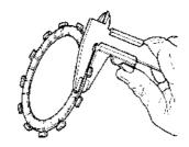
Measure the thickness of the plate across the friction material. Replace the plate when it wears by 2,7 mm/2,8 mm.
